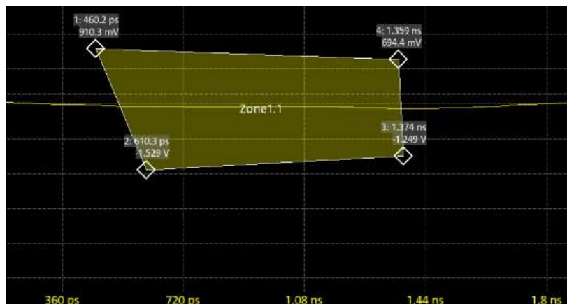
Figure 7-11: 1 area of a trigger zone
