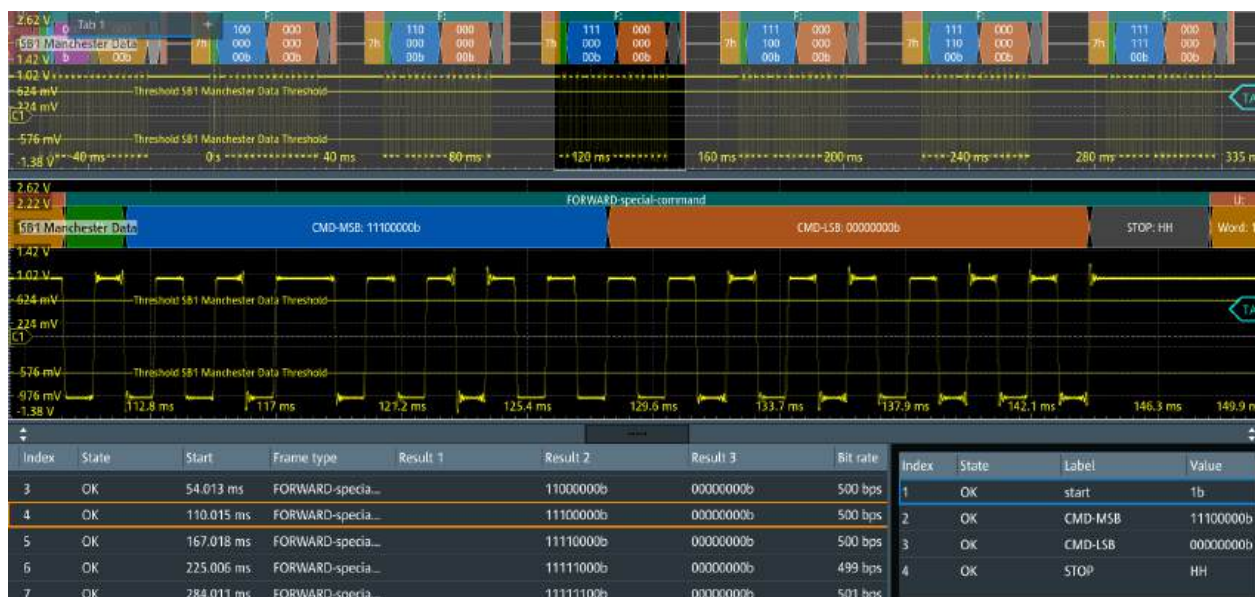
Figure 14-27: Decoded Manchester signal
