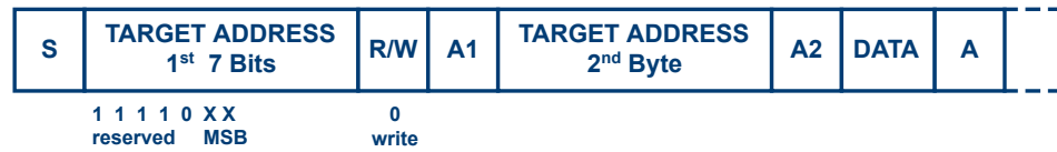
Figure 14-12: 10-bit address, write access
