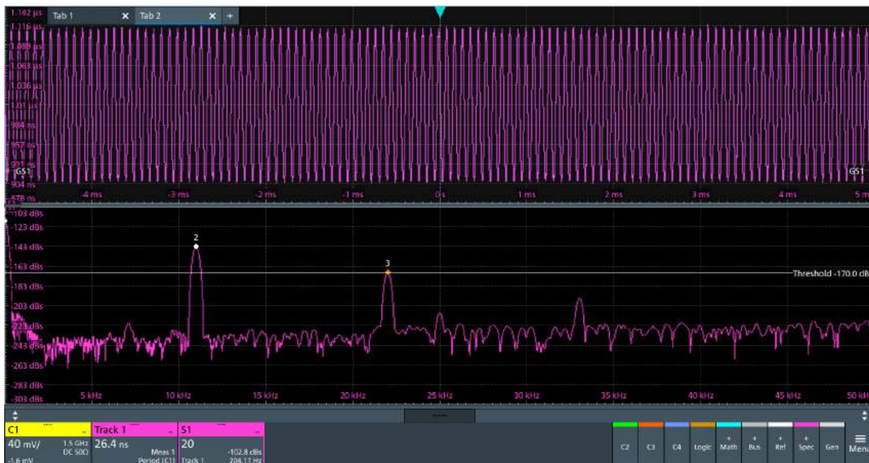
Figure 10-5: Track and spectrum on this track. C1 is not in the diagram.
